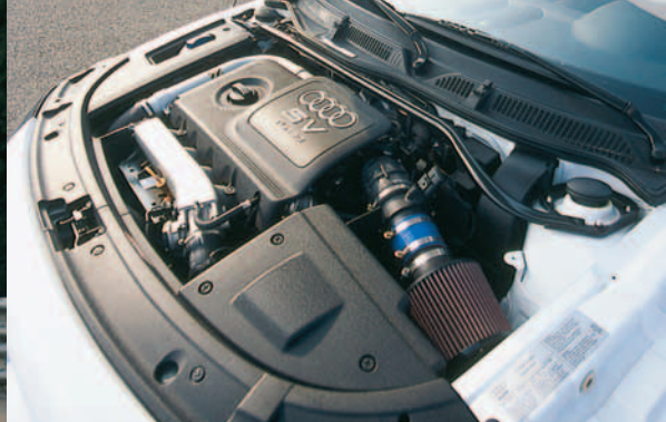
Under the hood sits the 225hp 1.8T with a GIAC chip and other PES goodies. Soon to be nestled there is PES's new Stage III, utilizing a Garrett T-28/T-35 turbo.
