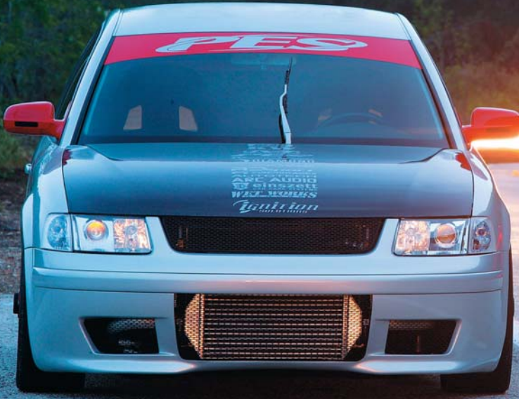
It's hard to miss the Spearco front mount intercooler jammed under the custom-trimmed front bumper.
