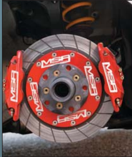
Femi fabricated the brackets to fit the dual MSR calipers to the 14-inch front rotors. Don't you hate Femi?
